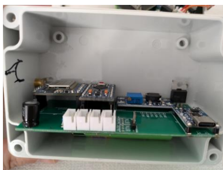
Figure 14 Installing the 15 board in the sensor box
