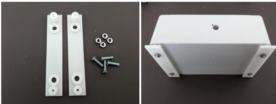
Figure 6 Attaching the mounting brackets to the sensor box
