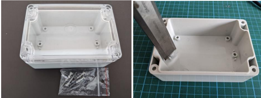
Illustration 4 Sensor housing, removing the nubs
