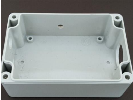
Figure 5 with drilling points (left) and finished drilled housing
